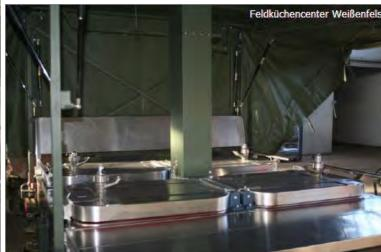
With TFK 250 two cooks can provide meals for 250 personnel or a single-course meal for 500 personnel in 2 hours. The trailer features swinging arm torsion bar suspension and is rated for cross-country movement with full boiling and frying pans.
