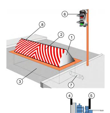
The hydraulic road blocker RSB76H was designed as an effective means of controlling access to high security areas (Impact resistance: theoretical K4 - 610KJ) such as embassies, airports, strategic factory sites, etc ...The RSB76H offers the advantage of not requiring a side column to house the drive mechanism.
